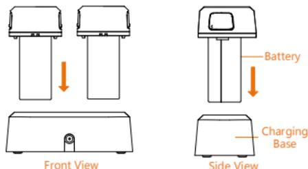
4. When the battery is fully charged, remove the battery from the charging station.
