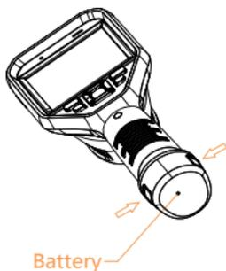
2. While holding the latches, pull out the battery socket to remove the battery as shown below.
