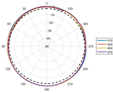
Azimuth (Top View): 698–960 MHz
